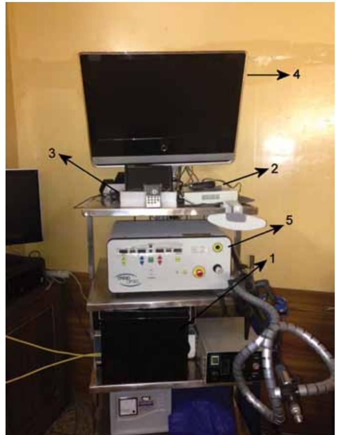
**Figure 2:** 3D PIP HDMI endoscopic visualization System. Black arrow 1:3D (Three Dimensional) PIP ( picture in picture) Endoscopic Visualization System. Black arrow 2: It is a Video recorder. Black arrow 3: It is a Remote Control for 3d PIP HDMI visualization system. Black arrow 4: LED Monitor. Black arrow 5: Endoscopic Unit.
