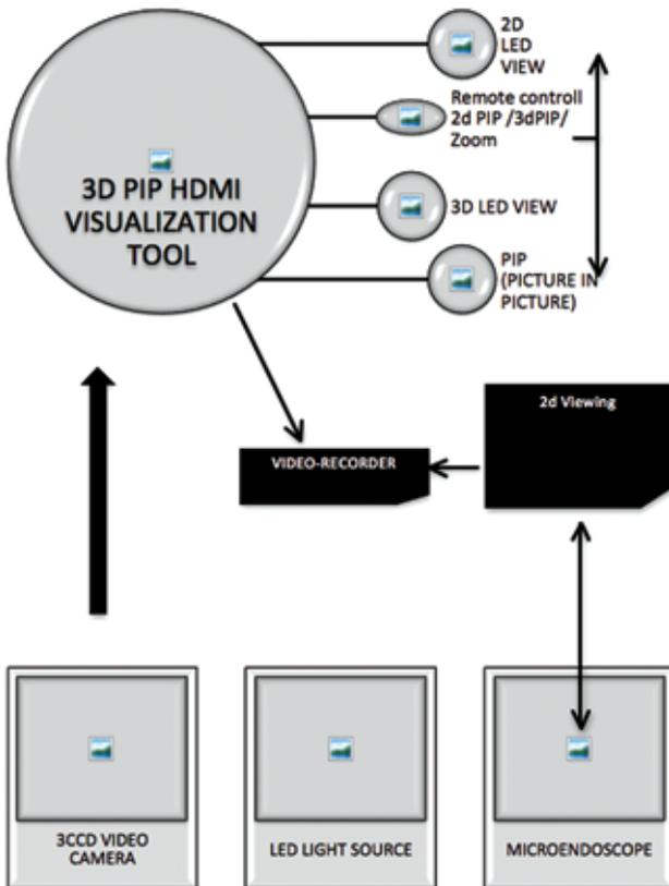
**Figure 1:** Diagrammatic view of 3d PIP HDMI visualization system and standard 2D Endoscopy system.
